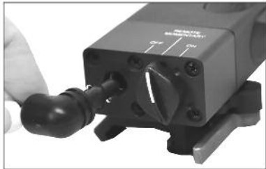
Figure 3-2 Remote Cable Switch Location
